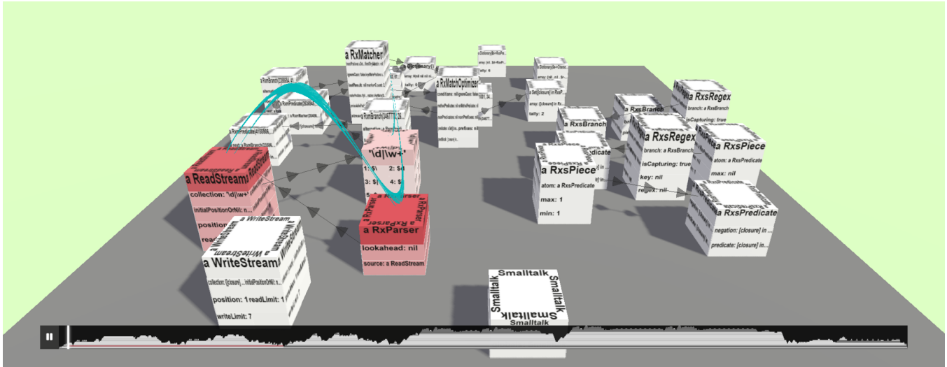
Figure 1: Screenshot of an animated object map showing a program trace for the construction of a regular expression matcher in the Squeak/Smalltalk programming environment. Blocks represent objects, arrows display references between objects, and color highlights and trails show object activations. The timeline at the bottom provides a temporal overview of the program trace and allows users to control the animation.
